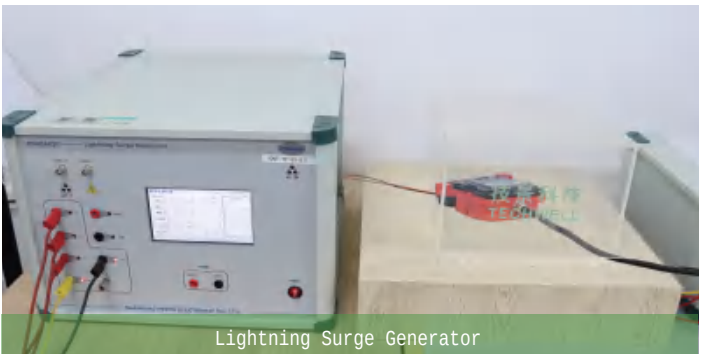
Lightning Surge Generator
