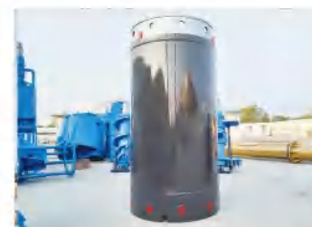
旋挖护筒 full casing
