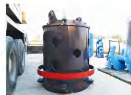
旋挖护筒 full casing
