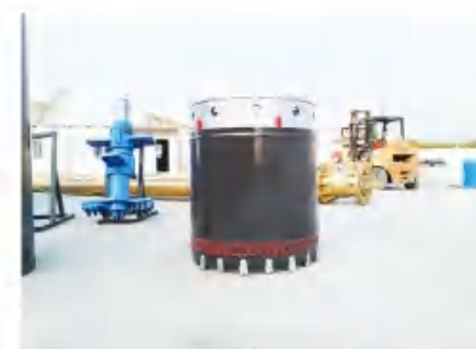
旋挖护筒 full casing
