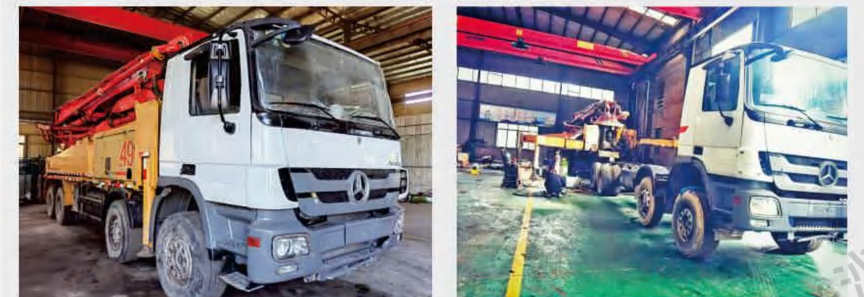
▲ Replacing the chassis, upgrading, and remanufacturing
