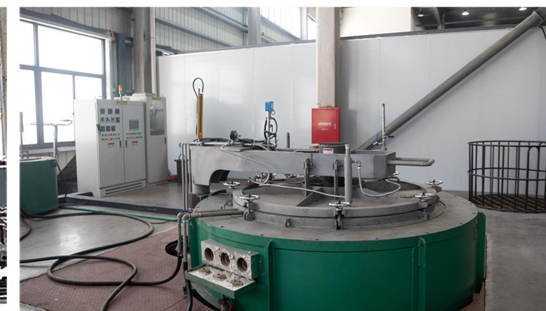
Nitriding furnace equipment
