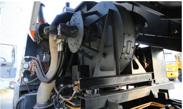
1.Efficient German centrifugal fan with energy efficiency up to 78%, Three-layer flow circulation design, minimum the dust, improve the suction.
