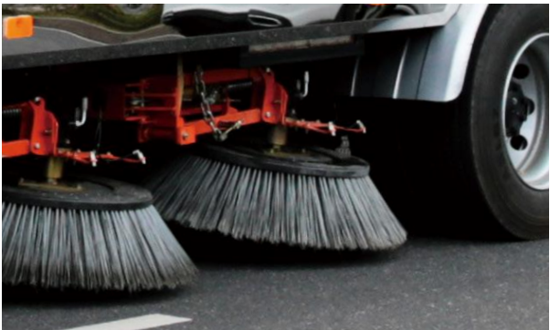
4.The central four-sweeping disc is used to achieve a sweeping width of 3800.
