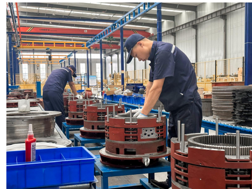
传动部件装配线 Transmission component assembly line
