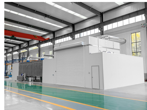
喷漆房 spray painting booth
