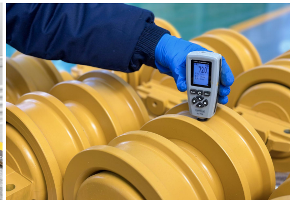
漆膜厚度检测 Measurement of Paint Film Thickness
