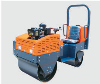
Model: HQ-YL700Z 1Tons Engine: Changchai 178F(4KW); Changfa 178F(4KW); Drum Width: Front 700MM, Rear 500MM; Weight: 1000KG;
