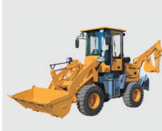
Model:HQWZ10-20 Engine:Yunnei YN25GB; Power:37KW; Bucket Capacity:0.1m³; Loading Capacity:0.5m³;
