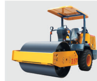
Model: HQ-YL3500 Engine: Changchai 390; Power: 39HP; Drum Width: 1200MM; Weight: 3500KG;
