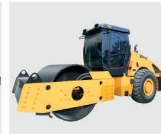
Model: HQ-YL26T Engine: Cummins B5.9CS4; Power: 154KW; Drum Width: 2130MM; Weight: 26000KG;
