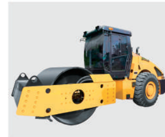
Model: HQ-YL20T Engine: WP6G190E301; Power: 140KW; Drum Width: 2100MM; Weight: 20000KG;
