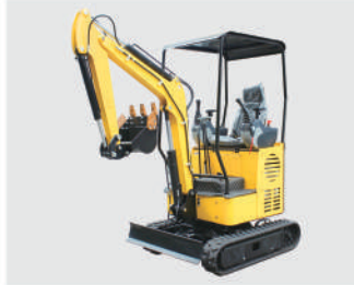
Model:HQ-17 Engine:Changchai/Kubota D722; Power:10.2 KW≈32PH; Bucket Volume:0.03m³; Weight:1700KG;
