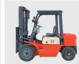
Model: HQ-3.5T Luxury Engine: XinChai; Rated lifting Capacity: 4300KG; Lifting Height: 3000MM; Vehicle Size: 2650*1260*2200MM;
