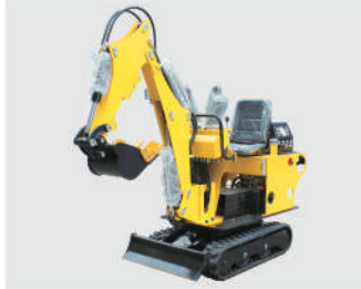
Model:HQ-08 Engine:Briggs&Stratton; Power:14HP; Bucket Volume:0.025m³; Weight:800KG;
