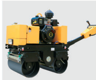
Model: HQ-YL800 Engine: Honda/CF186F; Power: 13HP/9HP; Drum Width: 635MM*2; Weight: 780KG;
