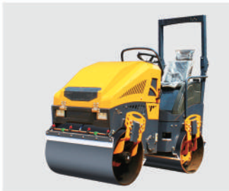
Model: HQ-YL1100Plus Engine: Kubota D1105; Power: 18.2KW/24.5HP; Drum Width: 1100MM *2; Weight: 3000KG;
