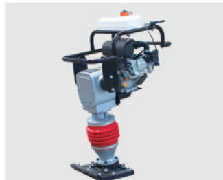
Model:HQ-D125 Engine:Loncin 168F Gasoline; Power:3.8KW/3600Rpm; Base Plate Size:480*550MM; Compaction Depth:350MM;
