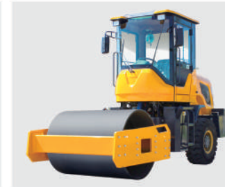
Model: HQ-YL4000 Engine: Yunnei 490; Power: 36.8KW; Drum Width: 1350MM; Weight: 4000KG;
