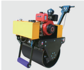
Model: HQ-YL700 Engine: Honda GX270(4KW); Changchai, Changfa 178F(4KW); Drum Width: 700MM; Weight: 500KG;
