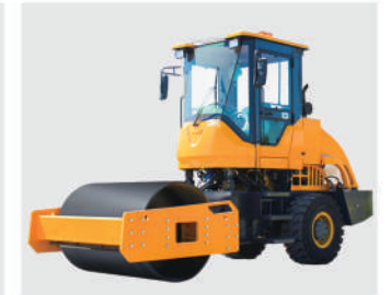
Model: HQ-YL5000 Engine: Yunnei 490; Power: 36.8KW; Drum Width: 1450MM(1400MM); Weight: 5000KG;
