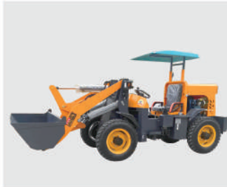
Model: HQ-909 Engine: Changzhou; Power: 25/28/30/32/35/38HP; Bucket Capacity: 0.35m³; Vehicle Size: 4000*1300*1450MM;
