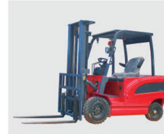
Model: HQ-1.5T-A Battery: Lead-acid; Battery Capacity: 70/100/200Ah; Rated lifting Capacity: 1500KG; Lifting Height: 3000MM;
