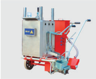
Model:HQ-HX100 Enhanced Version Coating Width: 100-450MM; Coating Thickness: 1.0-3.0MM; Machine Weight: 147KG; Vehicle Size: 1200*850*1200MM;
