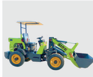
Model: HQ-910 Engine: Changzhou; Power: 25/32/35HP; Bucket Capacity: 0.35m³; Vehicle Size: 4000*1300*1600MM;
