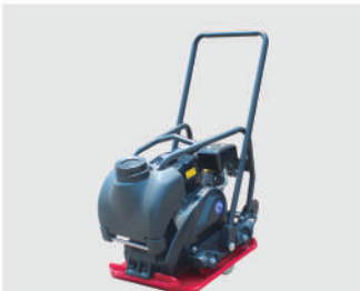
Model:HQ-C90 Engine:Loncin; Power:5.5-6.5HP; Base Plate Size:480*550MM; Compaction Depth:300MM;
