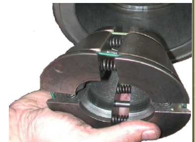
Forming head (Changing with tools) 模具更换需要工具
