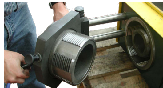
Forming head (Changing with tools) 模具更换需要工具
