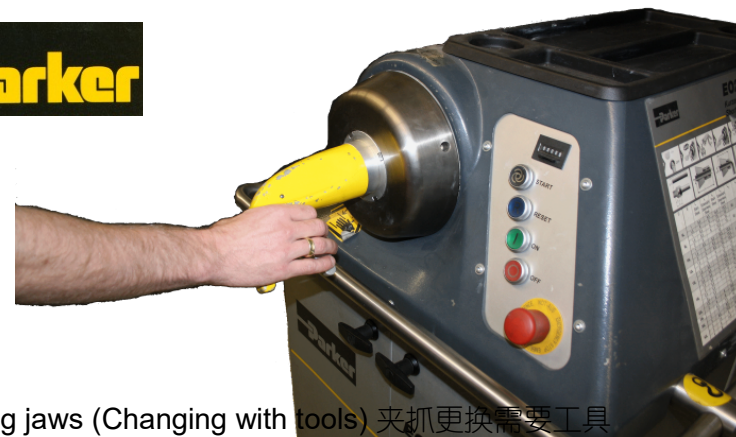
Forming head (Changing with tools) 模具更换需要工具
