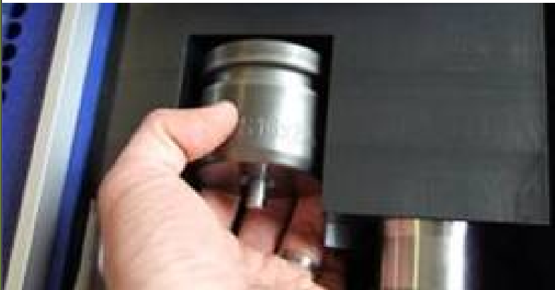
Forming head (Changing without tools) 模具更换不需要工具
