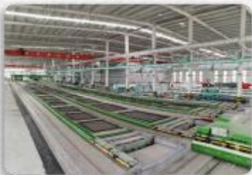
Prestressed Line 预应力生产线
