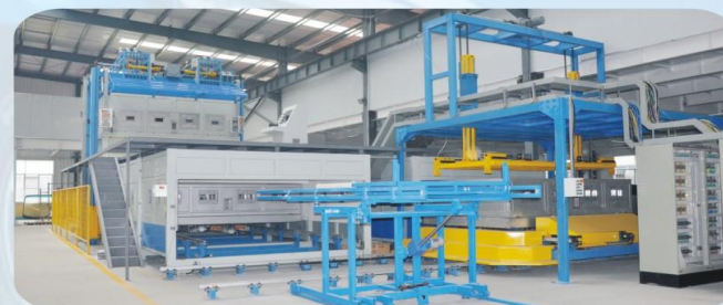
Continuous heat-bending furnace for bus front windshield and special oversized glass
