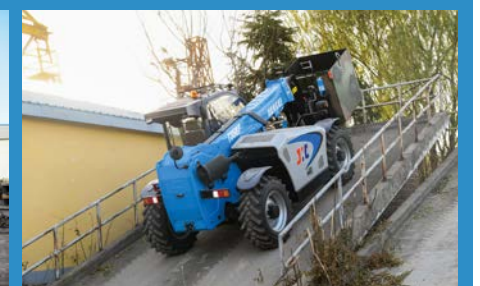
Max gradeability test at full load (45% slope)
