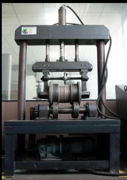
Wear tester simulates wheel travel to test wear conditions
