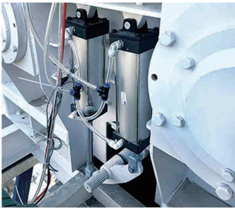
双气缸卸料 Dual-Cylinder Discharge System
