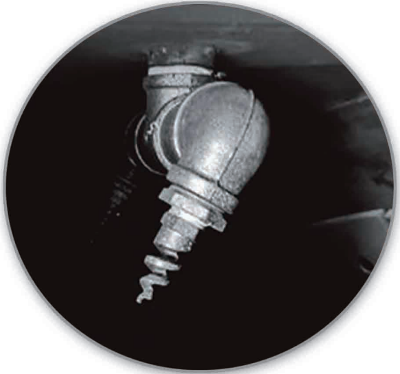
水路装置分为上置水路和内置水路解决了管路中残余外加剂和水现象 The water supply system employs both overhead and integrated piping, effectively eliminating residual admixtures and water retention in the lines
