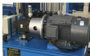
液压站 Hydraulic station
