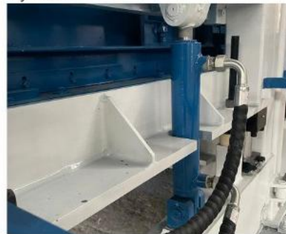
面料液压升降 Hydraulic lifting device for face material platform
