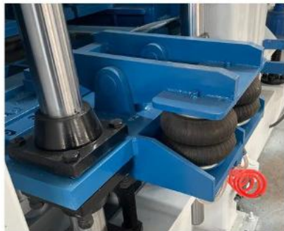
气囊夹紧系统 Airbag clamping for mould
