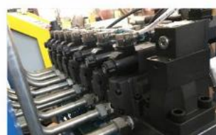
双油路液压系统 Double proportional + Single proportional hydraulic system
