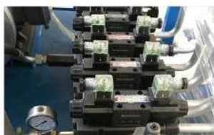
双回路液压系统 Double proportional + Single proportional valve hydraulic system
