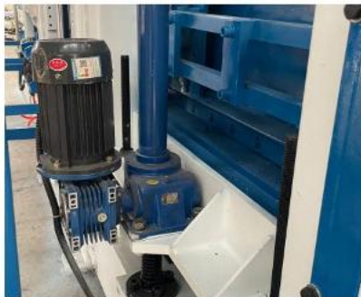
骨料电动升降 Electric lifting device for aggregate platform
