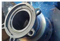
角焊缝气保焊
