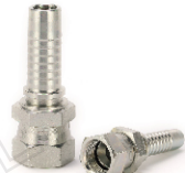
P26711D 美制JIC内螺纹74°内锥面双六角 JIC FEMALE 74° CONE SEAT DOUBLE HEXAGON SAE J514
