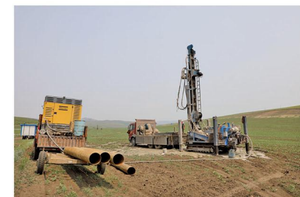
260m DTH drilling rig for irrigation in Philippine
