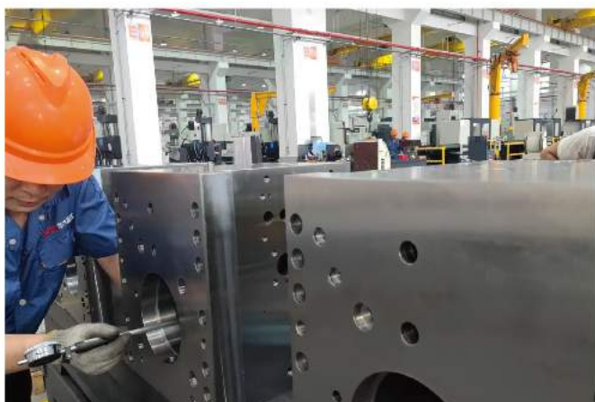
内径尺寸检查 Inner diameter inspection
