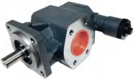
ZCB-C100-F2.5-L-E2-M1-JZ (ZCB-C series, displacement 100ml/r, with safety valve, set pressure 2.5Mpa, counterclockwise facing shaft, shaft head with rolling bearing, nitrile rubber seal, noise reduction process)
