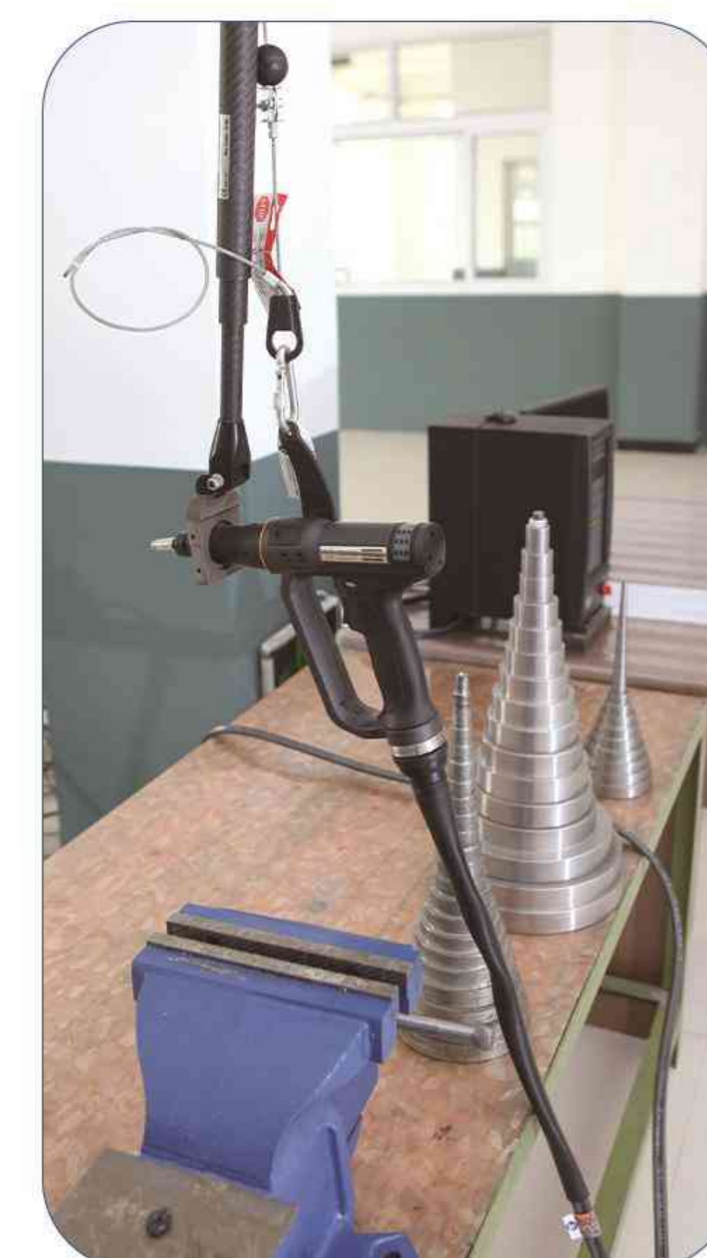
扭矩检测仪 To test the torque on basis of certain rotate speed
