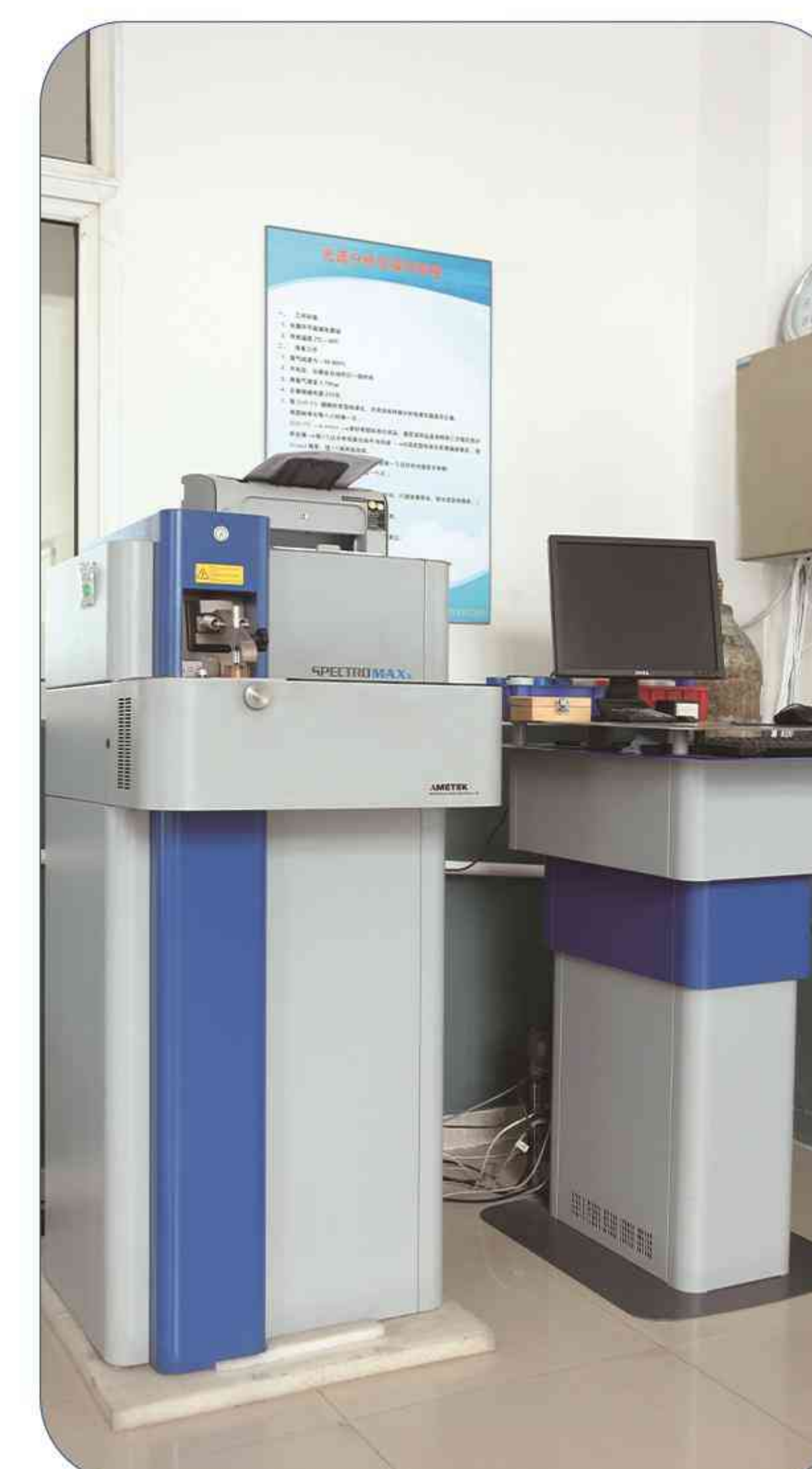
光谱仪 To test the composition of the raw material
