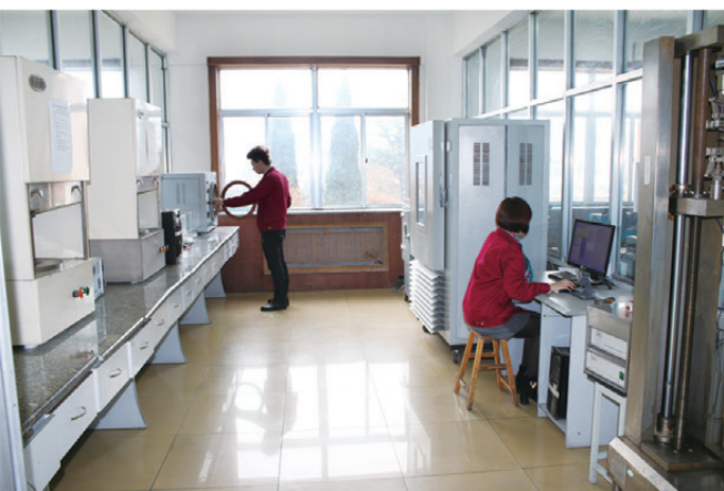
无转子硫化仪、门尼粘度仪、臭氧试验机、热空气老化试验箱等检测设备 Moving die vulkometer, Mooney viscometer, Ozone-resistance testing machine、 Hot air aging test chamber and other test equipments
