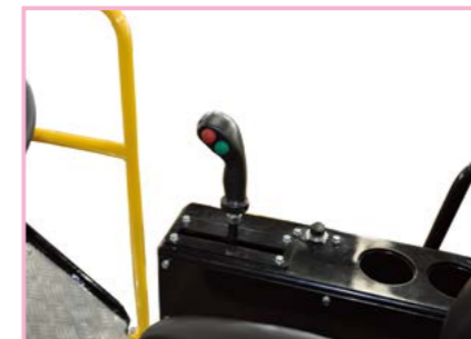
Walking reversing mechanism with a neutral locking function ensures safe start of the machine
