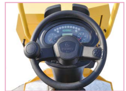
Integrated micro computer control plate, with operation, monitoring, alarm and other functions.
