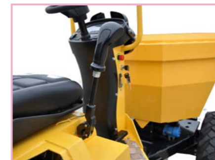
Walking reversing mechanism with a neutral locking function ensures safe start of the machine
