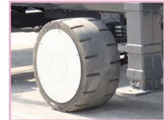
The solid tyre, puncture proof, long-life span
