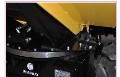
The hopper can rotate 270° and can be tilted forward, leftward, and rightward.
