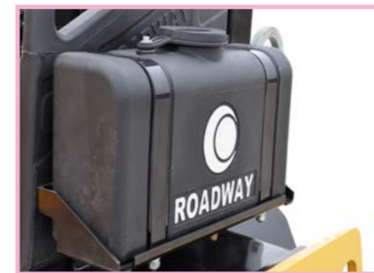
Emulsified liquid tank
