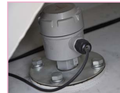
Set material level sensor in material box, control the feeding amount
