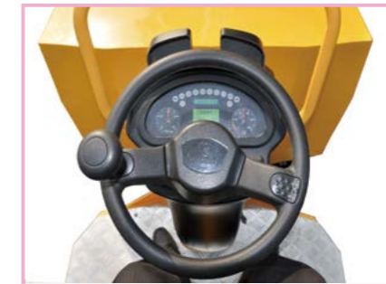
Integrated micro computer control panel
