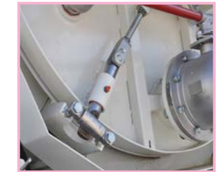
Four-point linkage lock mechanism
