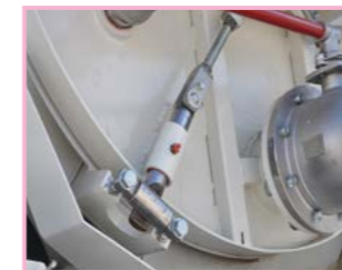
Four-point linkage lock mechanism
