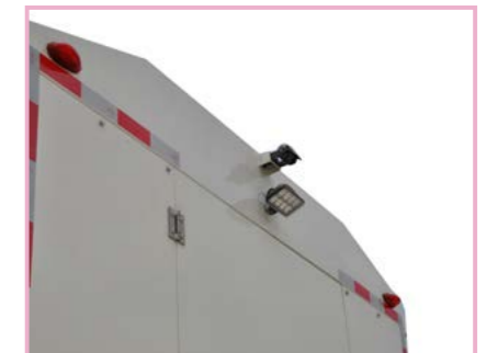
Install a camera, easy to observe the distribution of materials and obstacles behind the vehicle
