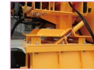
The mold hanged, dismantled hydraulically
