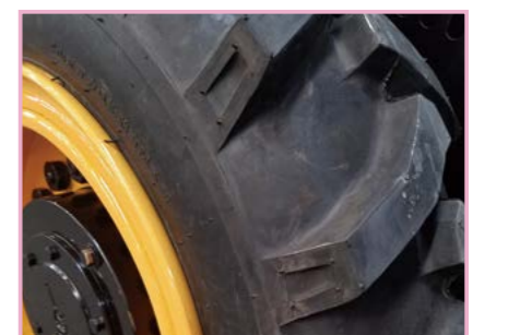
Herringbone tyre suitable for backfill construction
