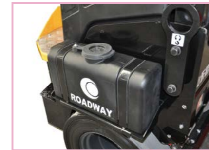
Emulsified liquid tank
