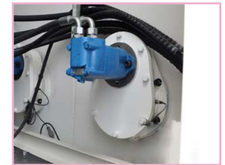
Spiral feeder equipped with Danfoss motor and gearbox, make the feeding more precise
