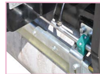
Stainless water-spraying pipe
