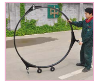
Cutting track with idler wheel, can transfer Easily.
