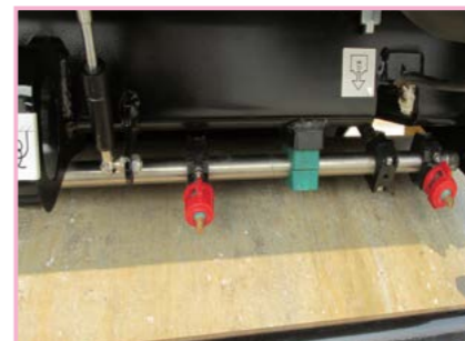
Electrically controller water-spray
