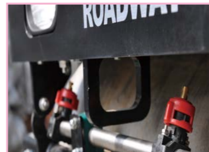
Electrically controlled water-spray, high efficient and water-saving
