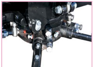
The articulated blade angle adjustable system, to make the angle on 5 blades are the same all the time
