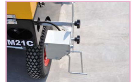
Automatic walking sensor, can correct direction, error within 1mm.
