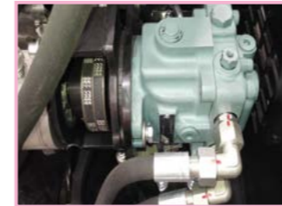
Imported Danfoss variable plunger pump drives the machine stepless speed walking
