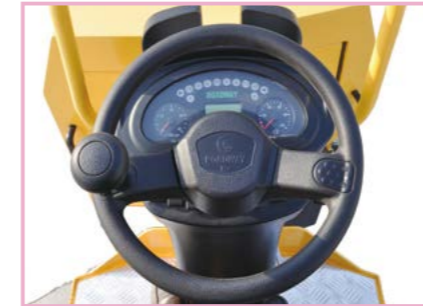
Integrated micro computer control plate, with operation, monitoring, alarm and other functions.
