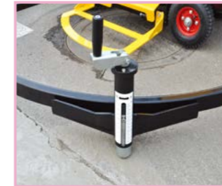
Cutting track with level indicator
