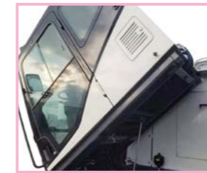
7. The cab can be tilted forward for easy maintenance
