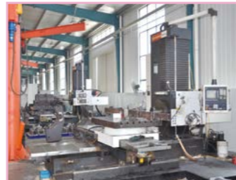
CNC boring machine
