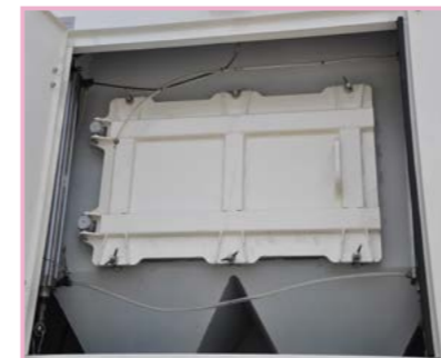
Set up four powder spreading gates to adapt to operations of different widths
