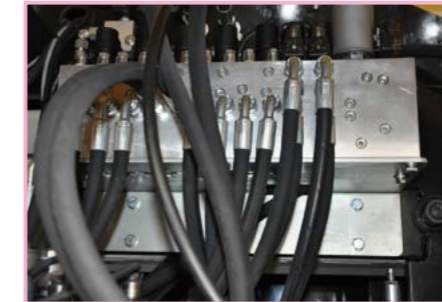
DANFOSS hydraulic system
