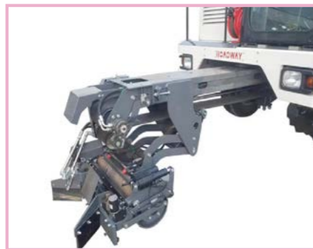
Paving and Compaction Part
