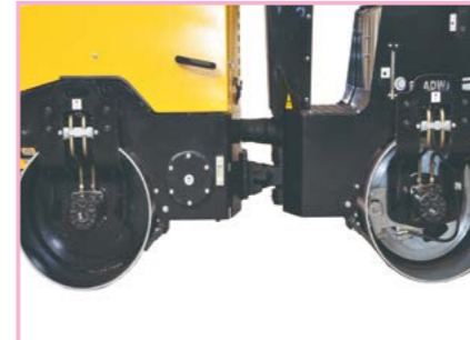
Double American brand cycloid hydraulic motors drive the machine walking
