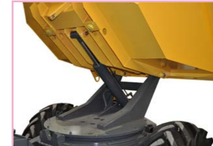
The hopper controlled by hydraulic cylinder
