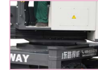
The machine can rotate 360°, specially designed soft start and stop
