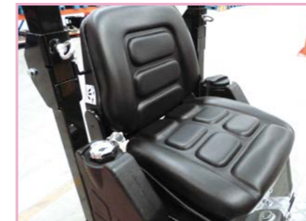
Seat with neutral start switch. Operator sits up, the engine will stop.
