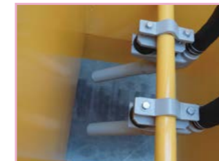
Hydraulic vibrating rod
