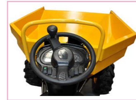
Integrated micro computer control panel, which can realize various functions such as operation, monitoring and alarm
