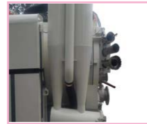
Twin channel cyclone separator
