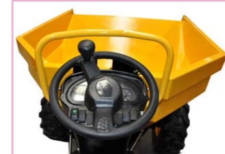
Integrated micro computer control panel, which can realize various functions such as operation, monitoring and alarm
