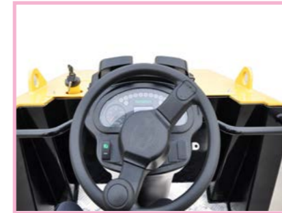
Integrated micro computer control panel
