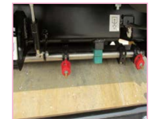
Electrically controller water-spray
