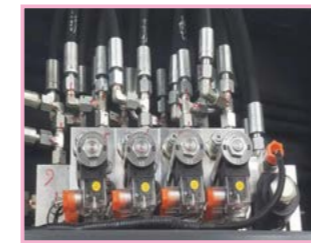
5. Hydraulic Control Valve set with SUN, Hy-draforce Valve element
