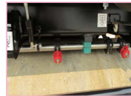
Electrically controlled water-spray, high efficient and water-saving
