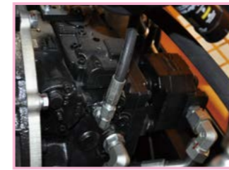
Imported hydraulic variable plunger pump, drives the machine stepless speed walking
