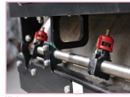
High-pressure water spray system, sprinkler nozzle can be quickly replaced
