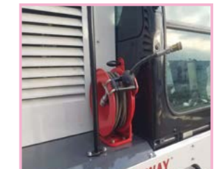
12. With high-pressure cleaning liquid spray gun
