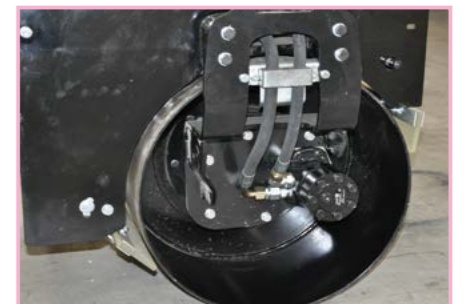
American brand hydraulic motor, drive the front drum walking
