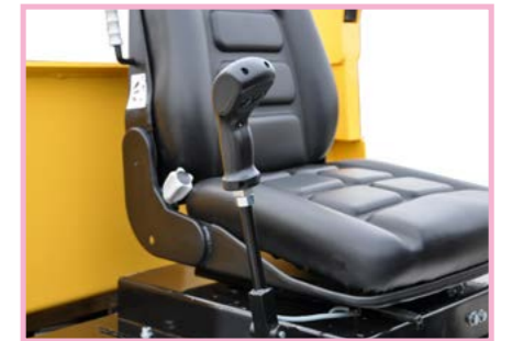
Walking reversing mechanism with a neutral locking function ensures safe start of the machine
