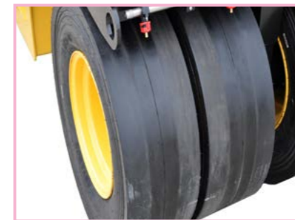
Wide-base smooth tyres, which can compact asphalt densely
