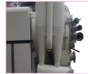
Twin channel cyclone separator
