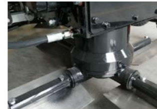
Blade angle adjustment mechanism is hydraulically controlled and with sealed cover without cleaning
