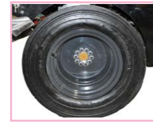
Wide-based smooth tyres, which can compact asphalt and concrete road, and can also compact viscous, and sandy base materials.
