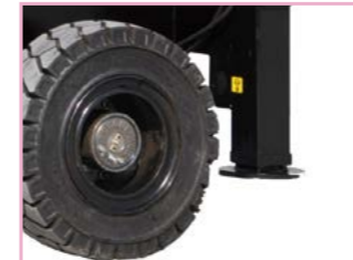
The solid tyre, puncture proof, long-life span
