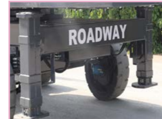
Hydraulic supporting legs, one-key leveling
