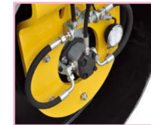
Danfoss hydraulic vibration motor
