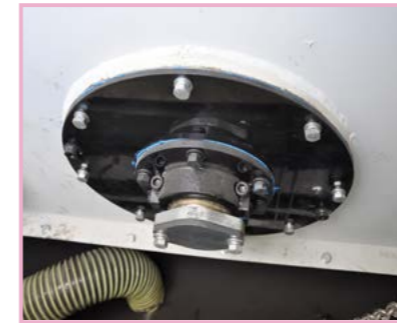
The bearings of the spiral feeder are protected by multiple high-pressure shaft seals, long service life
