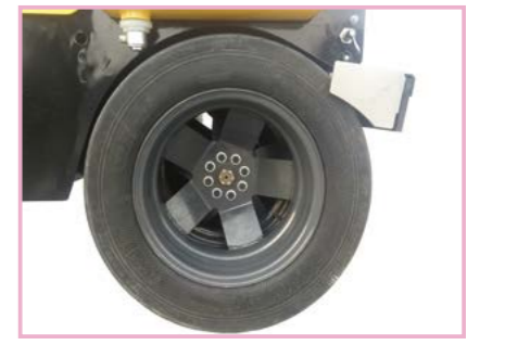
Wide-base smooth tyres, which can compact asphalt and concrete road, and can also compact viscous, and sandy base materials.
