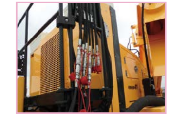
Italy brand quick plugs for external connections
