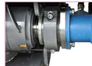
The auger bearings are seal designed, forbidden the concrete seeping in
