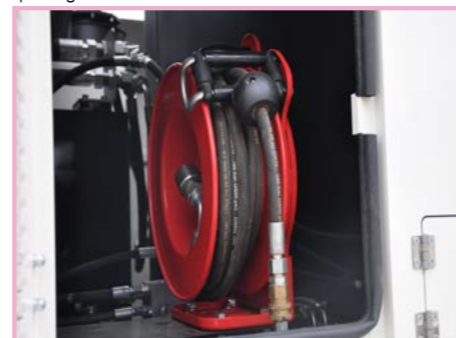
With high-pressure emulsified asphalt spray gun
