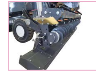
The screed head can turn upward, easy to clean
