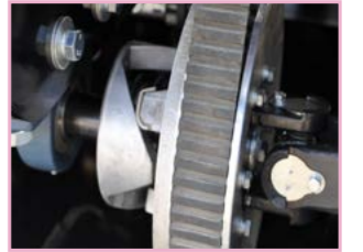
Stepless speed, clutch wheel to change the speed from very slow to very fast easily
