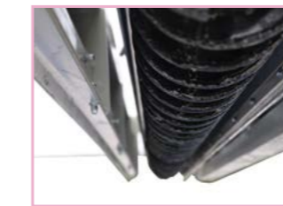
Specially designed auger, the dynamic balance is excellent, improved the leveling accuracy
