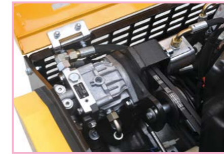
American light-duty variable plunger pump drives the machine stepless speed walking
