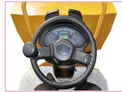
Integrated micro computer control panel
