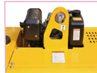
Lifting point for the convenience of lifting
