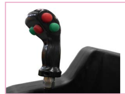
Forward/reverse running and vibrating all controlled by the integrated control lever
