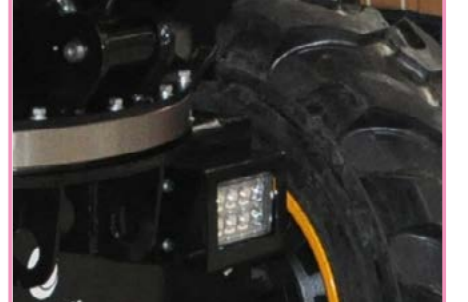
With LED high-intensity lighting for night construction
