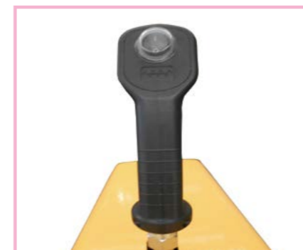
Forward/reverse running and vibrating all controlled by the integrated control lever
