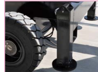
Hydraulic supporting legs one-key leveling
