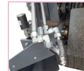
10. With high-pressure air cleaning and emulsified asphalt nozzle
