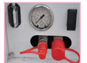
Hydraulic power interface for other hydraulic tools
