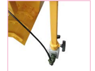
High sensitivity tilt sensor, to control direction
