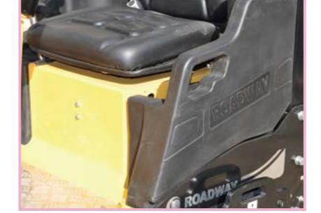
Plastic water tank free from corrosion and convenient for the water-spraying
