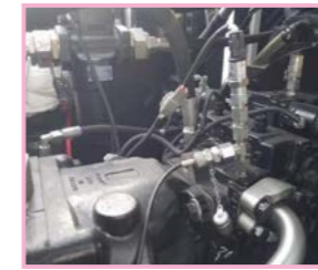
2. Danfoss hydraulic pump and hydraulic motor
