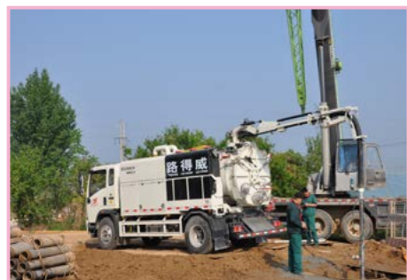
The machine is sucking up mud at the construction site
