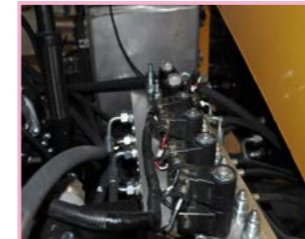
Hydraforce hydraulic integrated valve group
