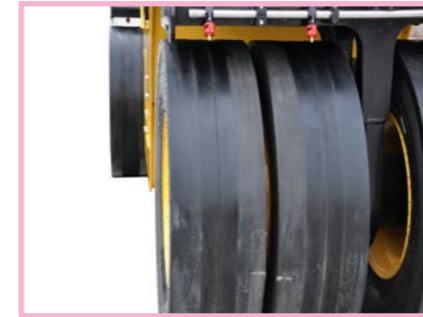
The front and back tyres are staggered, which make compaction completely
