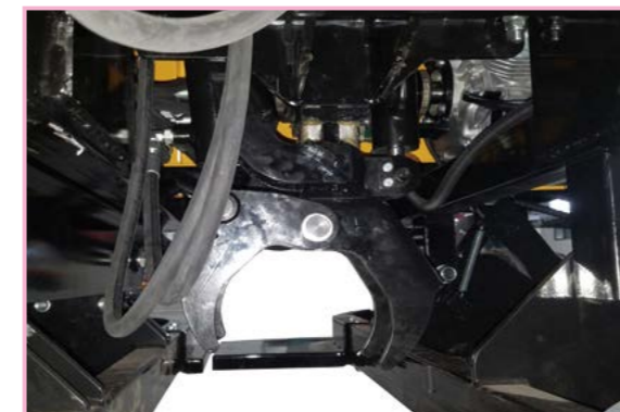
The conveyer pipe picked up automatically by hydraulic
