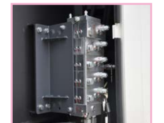
12. Hydraulic Control Valve set with SUN, Hy-draforce Valve element
