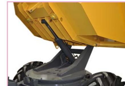
The hopper controlled by hydraulic cylinder
