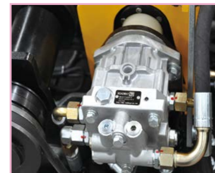
American light-duty variable plunger pump drives the machine stepless walking
