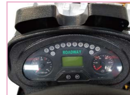
Integrated micro computer control panel
