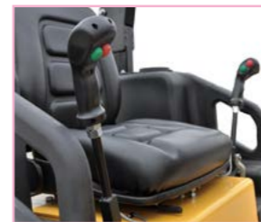
Walking reversing mechanism with a neutral locking function ensures safe start of the machine
