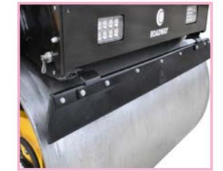
Super wear-resistant scraper, which can be picked up when transition
