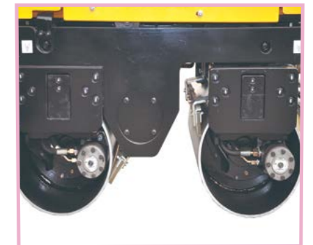
Double American brand cycloid hydraulic motors drive the machine walking
