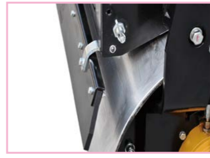
Super wear-resistant scraper, which can be picked up when transition
