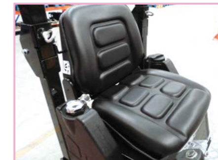
Seat with neutral start switch, operator sits up, the engine will stop.
