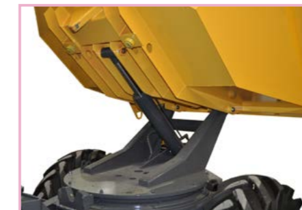
The hopper controlled by hydraulic cylinder
