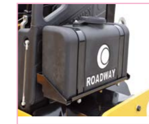
Emulsified liquid tank
