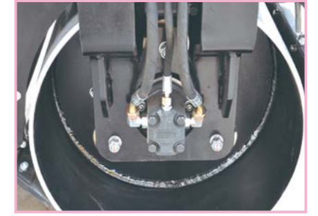
Steel drum vibrating is driven by imported motor and button controlled
