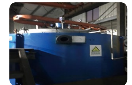
氮化炉 Nitriding Furnace
