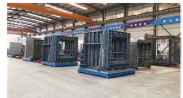
管廊模具制作现场 Manufacturing Site
