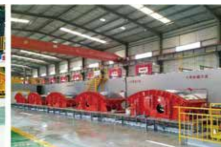
中铁四局集团 1+4 管片生产线 China Railway 4th Bureau 1+4 Segment Carousel
