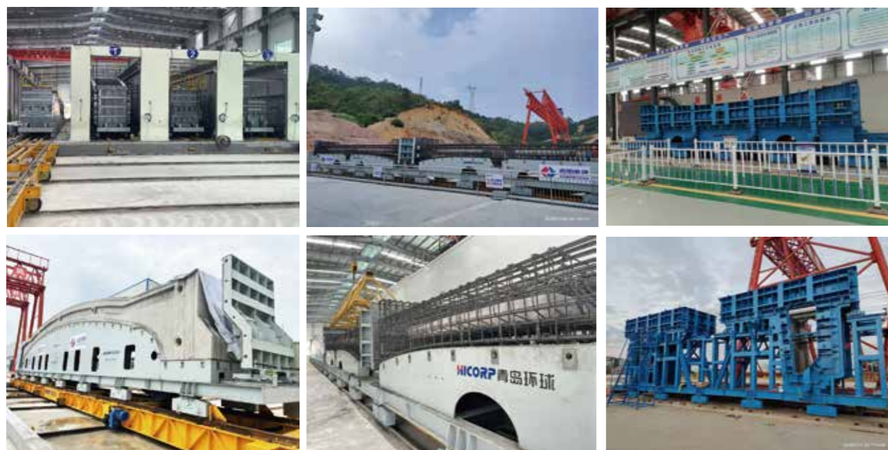
装配式地铁站生产线 Prefab Station Component Production Line
