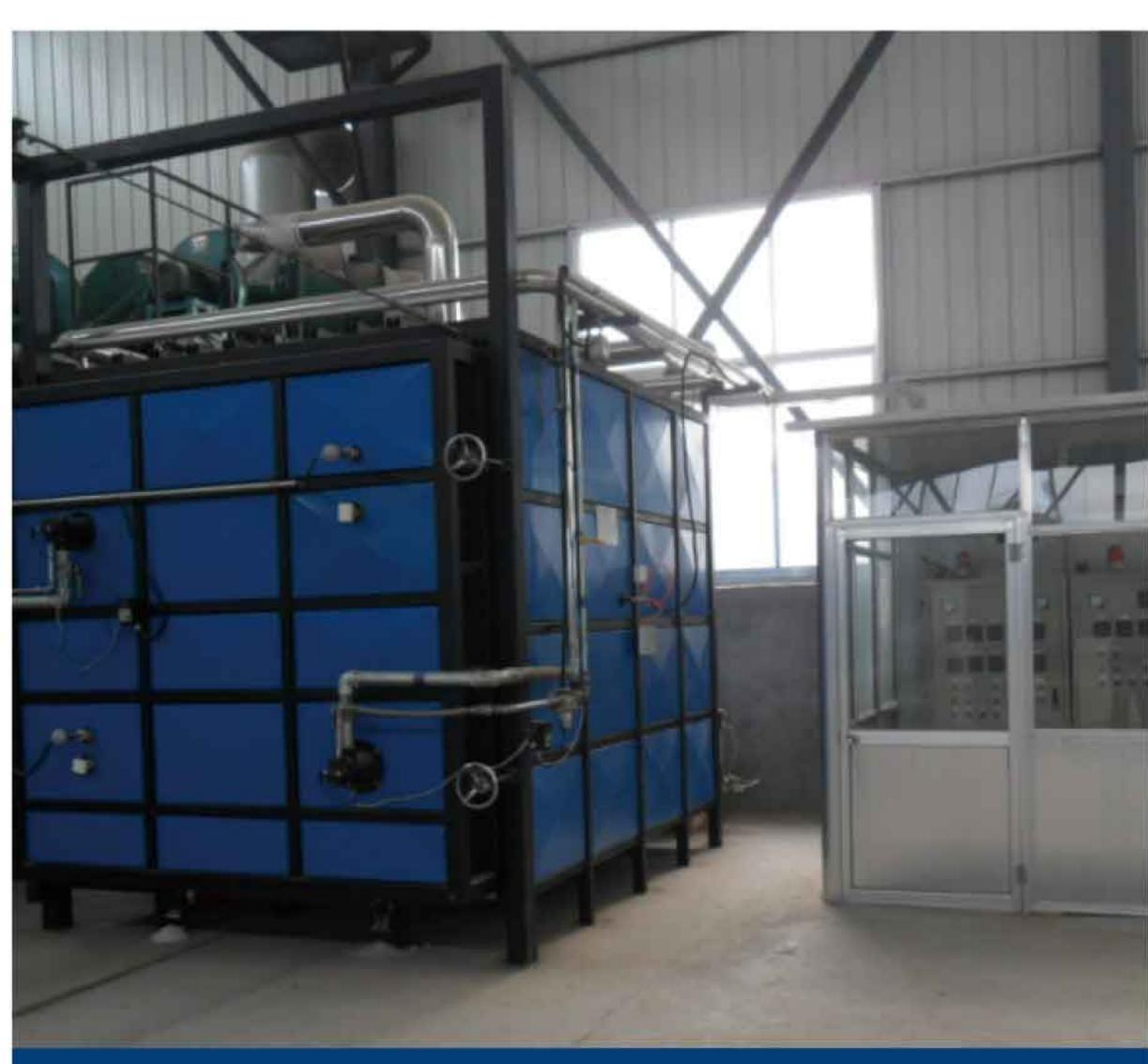
Pin shaft tempering equipment: After high-frequency and intermediate frequency, the pin shaft must be tempered through the equipment to eliminate the internal stress of the quenched workpiece, stabilize the production organization, and improve the overall quality.
