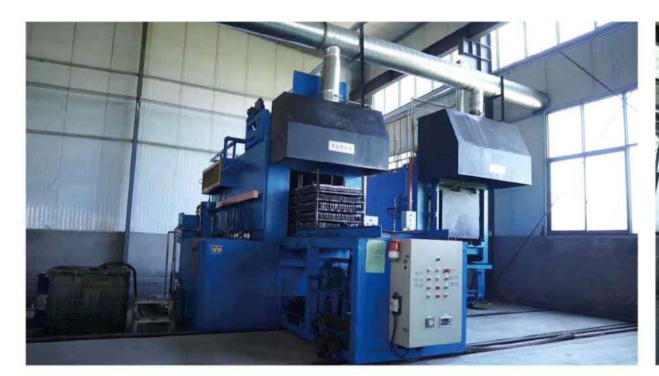
The box type carburizing furnace is a fully automatic production line composed of a heating greenhouse, an oil cooling chamber, a cleaning chamber, and a tempering chamber. This equipment is specially prepared for lining heat treatment. The carburized product has extremely stable carburization depth and hardness, and minimal deformation, greatly reducing the stability of the grinding process. The carburization depth can reach 0.8MM-1.6MM, HRC55-62.
