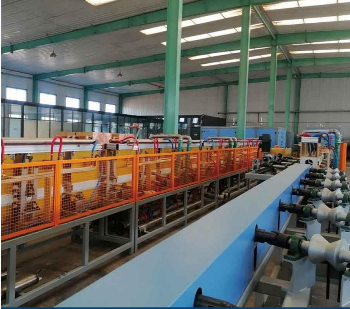
Pin shaft quenching and tempering production line: Adopting advanced quenching and tempering production line, HB Brinell hardness is stable, quenching and tempering depth meets national standards, and quenching and tempering organization standards can reach 2-3 levels.
