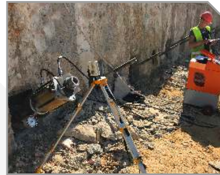
Load sensor Atlant and hydraulic Jack for ground anchor testing
