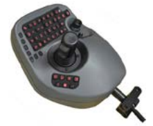
WP: Operator Control Module
