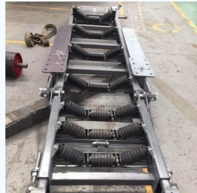
车载皮带机 Carried Belt Conveyor
