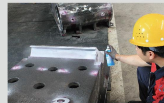
渗透探伤 Penetrant testing
