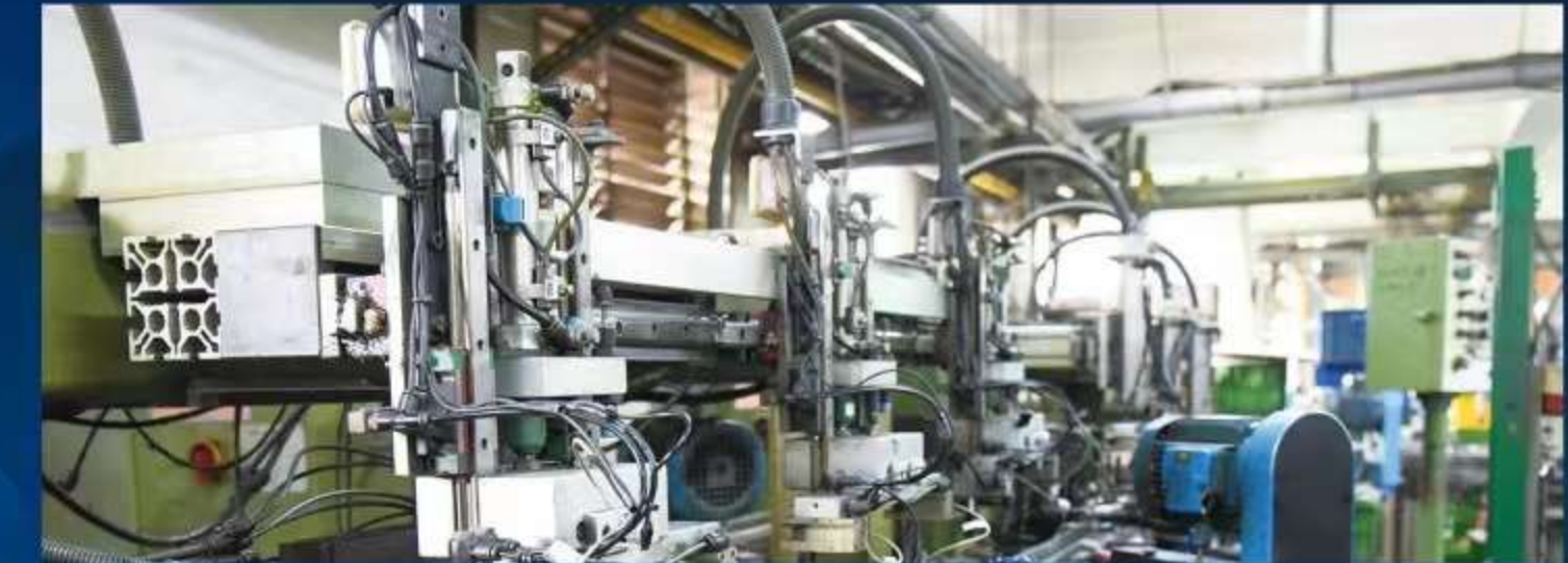
Fully automatic bearing production line (From Miba, the bearings supplier to Mercedes Benz & BMW)
