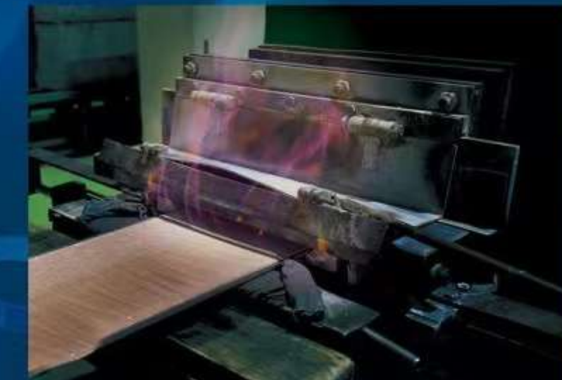
Bimetal bearing material sintering furnace
