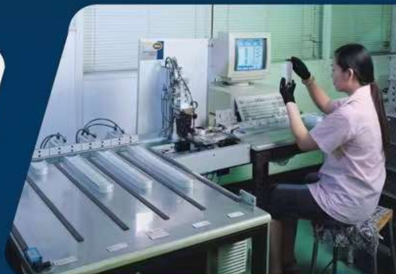
100% Bearing wall thickness inspection (auto)
