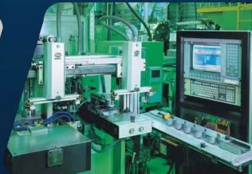
Online 100% inspection for bearing crush height
