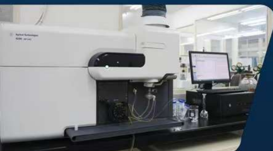
Inductively Coupled Plasma(ICP). Analyzing chemical composition
