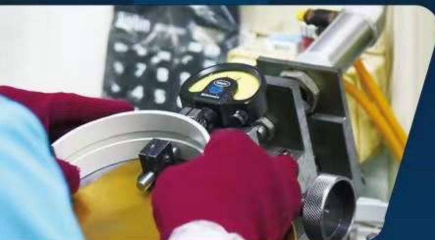
100% Bearing wall thickness inspection
