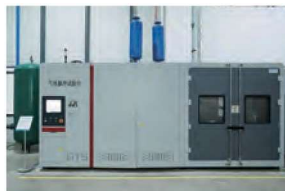
Air Pressure Pulse Test 气脉冲试验
