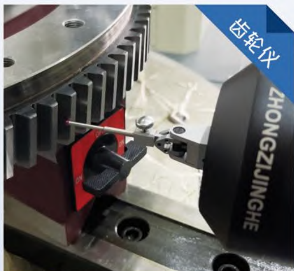
GEAR TESTER DETECTION
