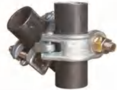
PZ-C13 德式旋转扣件 German Type Forged Swivel Coupler 48.3mm 1.45kg
