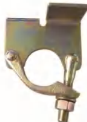
PZ-C10 固板扣件 Forged Board Retaining Coupler 48.3mm 0.6kg
