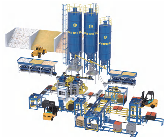
▲ Single Line + Online Cubing System
