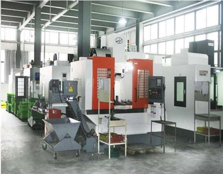
CNC Centers (65sets) Max. length: 1200mm Min. tolerance: 0.01mm
