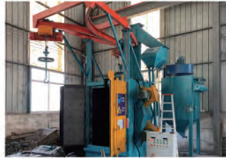
抛丸机 Shot Blasting Machine
