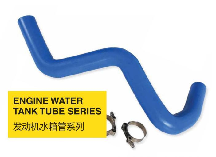
Used in engine cooling system, Bright Wind system, air delivery system, material: EPDM, polyester reinforced layer, working temperature:-40°C  $\sim$  150°C, working pressure: 0.5 mpa  $\sim$  1.0 mpa.
