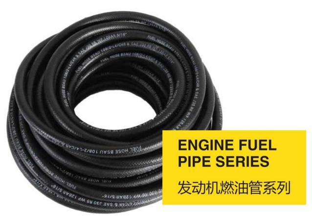
Used in engine fuel EFI system, oil delivery system, gearbox oil cooling system, intake breathing system, material:FKM, ECO, NBR, polyester reinforced layer, working temperature: -40°C ~ 150°C, working pressure:10mpa ~ 25mpa.
