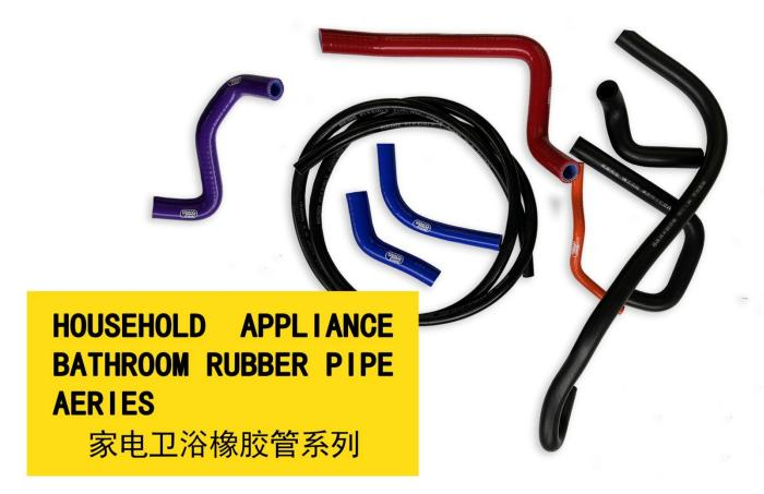
Applied to the transmission of water pipes, drainage pipes, heating pipes, etc. on smart home appliances and smart bathroom products Delivery system, material: EPDE/silicone, working temperature:  $-50~^{\circ}\text{C}^{\sim}150~^{\circ}\text{C}$ , working pressure:0.3mpa^2.0mpa.
