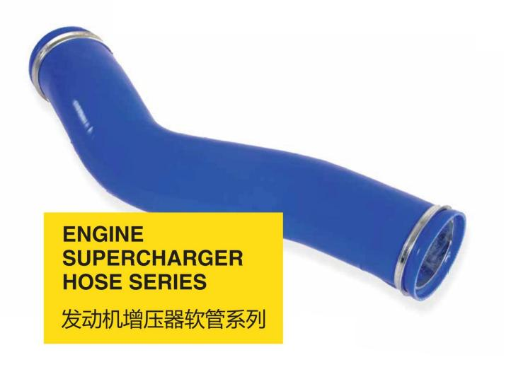
Widely used in mechanical engine turbocharger intake system, material: silicone rubber, amid reinforced layer, working temperature:- $50^{\circ}$ C ~  $250^{\circ}$ C.
