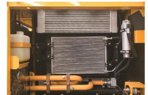
The hydraulic oil radiator, water radiator and inter-cooler are placed horizontally in parallel, which is effective in heatdissipation and easy to clean.
