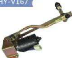
PC200-7 20Y-54-39442-52211 雨刮电机 Wiper Motor
